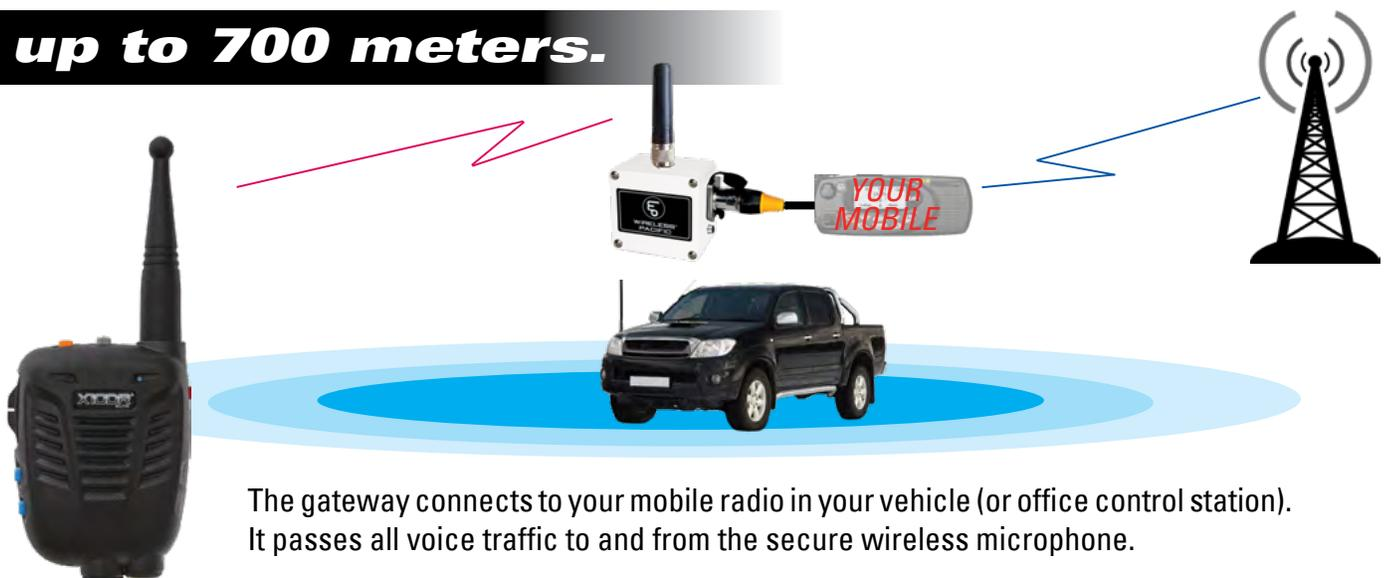
The gateway connects to your mobile radio in your vehicle (or office control station). It passes all voice traffic to and from the secure wireless microphone.
